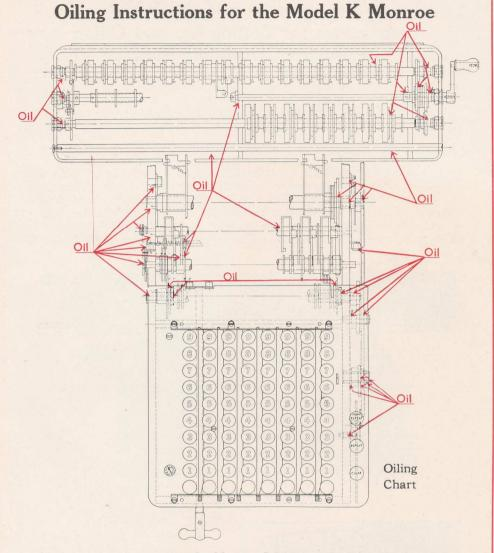
When in continuous use, the Monroe Calculating Machine should be oiled monthly. When used periodically, it should be oiled once every six weeks or two months.
