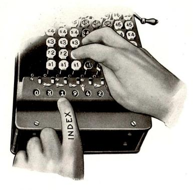
This stroke on the keys reduces the remainder to 19, which is smaller than the divisor. Were it still larger, we would continue to strike until the remainder became smaller than the divisor.
