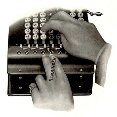
figure in the next column to the left changes to 2, as shown in above cut. Therefore, strike another time. On the second stroke the number of strokes made on the keys (two) agrees with the figure 2 in the next column to the left, and we observe that our remainder, 40, is less than the divisor 77.
