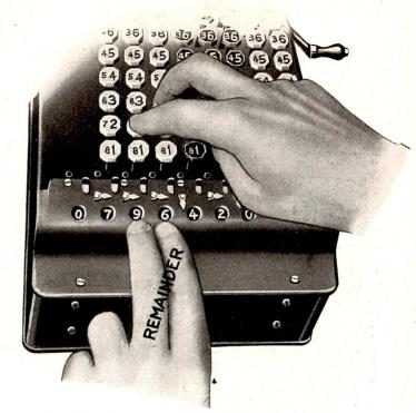
Press these keys representing the divisor repeatedly while counting the strokes out loud until the number of strokes made agrees with the figure standing in the register in the next column to the left of those on which the keys are being struck. See cut on opposite page where this figure is a "6" and is marked "Index."
