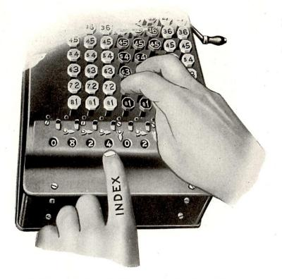
In this position the next figure in the column to the left of the keys on which the fingers rest is 4, as shown in above cut. Therefore, we depress the divisor while counting out loud: "one," "two," "three," "four." As the four did not change to a five, or any higher figure, the number of strokes on the keys now agrees with the figure in the next column to the left
