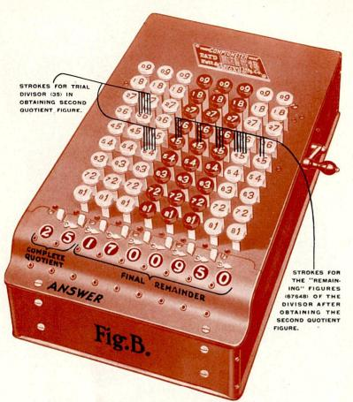
Again using the two left-hand figures as a trial divisor we find that the second quotient figure is 5, so put the right-hand finger on the large 5, one column to the right and count: "six, seven, eight," move to the right and count: "seven, eight," and so on for each of the remaining figures of the divisor, when pointing off we have 25 + 1700950. See Fig. B.
