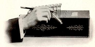
To Set the Machine at Naught, Give the lever on the right of the machine a full back and forward stroke.
