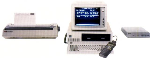
Psion Organiser II has a standard peripheral port at the top of the machine to allow a wide variety of devices to be attached for communications and specialized applications. Once the peripheral has been connected, additional commands which access the codes from the peripheral are activated automatically within Organiser II.
