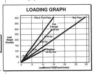
Now let's see...do we have the weight and CG information that we need? Well, for the front seats, the loading diagram shows an arm of 37 inches, and the loading graph shows min and max weights of zero and 400 pounds. Fine. We'll use 200 pounds for the mid weight.
