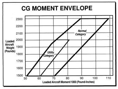
Unfortunately, Cessna's old POH format provides only a "CG moment envelope" so we have to calculate the "CG arm envelope" for ourselves. To do this, we locate each "corner" of the moment envelope and calculate the CG arm by dividing the moment by the weight (just as before).
