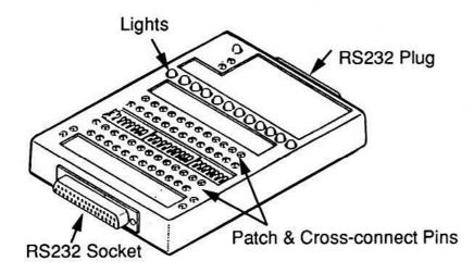
There will be some patch wires supplied with the BOB and you may also get an RS232 extension cable with 25 way serial plugs/sockets on either end.
