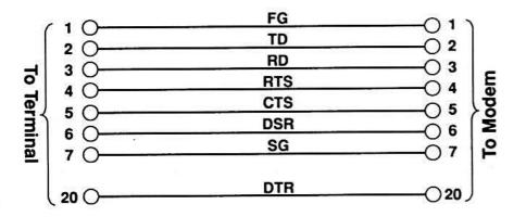
All the wires apart from Frame and Signal Ground are 'paired up' by function. Each wire in a 'pair' handles the same type of signal but in different directions. For example RD and TD (these are sometimes known as TxD and RxD), TD carries the outgoing data while RD carries data going the other way. Other 'pairs' are RTS/CTS and DTR/DSR.
