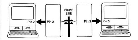
When two of the same are talking to each other RD on one should be wired to TD on the other, RTS should be wired to CTS, and DTR should be wired to DSR.
