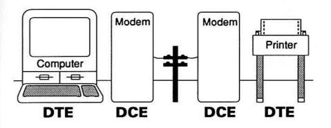
The RS-232 standard makes the wiring between a DTE (a computer or terminal) and a DCE (a modem) the easiest to configure because the wires go straight across. Pin 2 on the computer connects up with pin 2 on the modem's RS-232 port.
