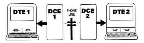
one modem (DCE1) will be transmitting while the other (DCE2) will be receiving. If the data is being transmitted on pin 3 it will be picked up by DCE1 on its pin 3. But on the other side of the telephone line DCE2 will pick up the signal on its pin 2 and it will then go to DTE2's pin 2 as well.
