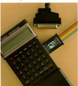
The software pack contains the programs which control the flow of information to and from the ORGANISER. Once the programs have been set, the software pack is replaced by a datapak to transmit or receive information through the connector pack.
